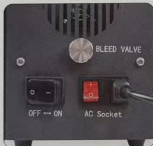
5 Start the power supply and start the electric air pump.
