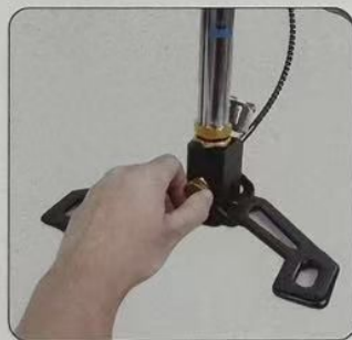
5 Unscrew the pressure relief valve of the air pump until the pressure gauge pointer of the air pump reaches zero.
