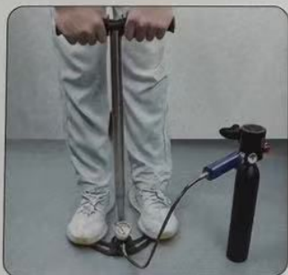
4 Stop air inflation when air pressure reaches 3000psi or 200bar.
