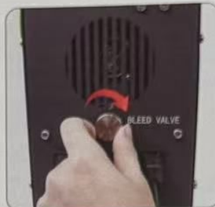
3 Ensure that the bleed valve on compressor is closed.
