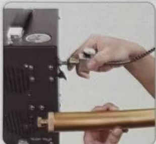
1 Screw the Compressor Refill Adapter onto Refill Port.
